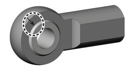
Figure 7: Lubricate cable rod ends with silicone spray lubricant Important: Do not use petroleum-based lubricants.
