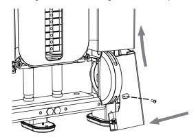
Figure 11: Installation of corner cover
