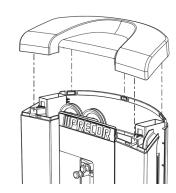
Figure 17: Shroud top cover attachment
