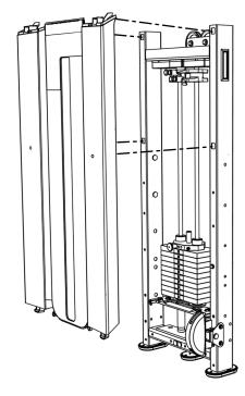
Figure 9: Front shroud attachment
