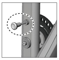
Figure 9: Lubricate the pop pin by pulling it out
