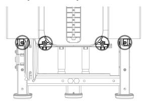
Figure 10: Screw locations on the front shroud
