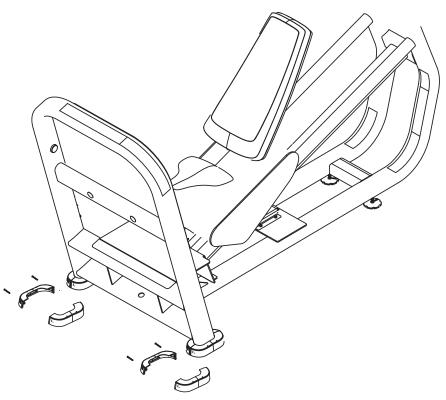
Figure 4: Foot cover positioning
