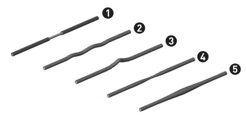
Figure 2: Signs of cable damage
