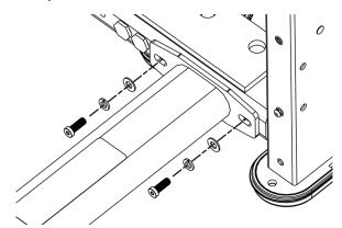
Figure 19: Remove bottom bolts from the weight tower
