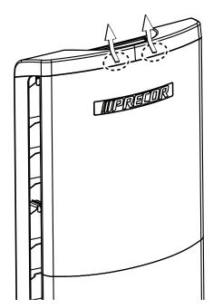
Figure 1: Removing the Top Cover
