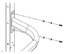
Figure 18: Remove side bolts from the weight tower
