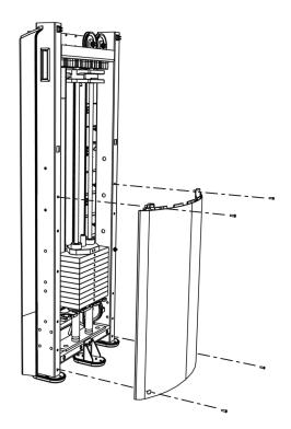
Figure 15: Lower back shroud attachment
