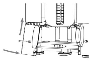
Figure 13: Tab slides under the front shroud
