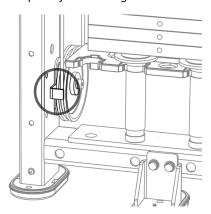
Figure 20: Thread cable inside the hook
