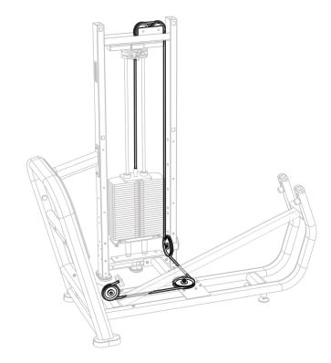
Figure 21: Cable rerouting
